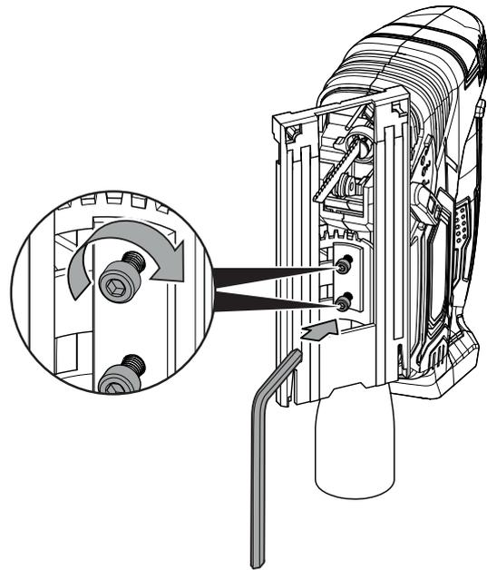
8. Check the base plate (6) for tight fit.
