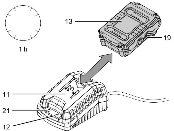
2. Insert the mains plug of the quick charger (11) into a properly fused mains socket.
