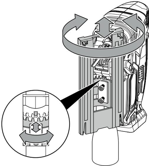
5. Set the desired cutting angle. The number of degrees to be set is engraved on the base plate (6).
