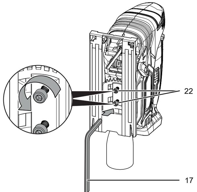
4. Slide the base plate (6) to the rear until it can be freely rotated.
