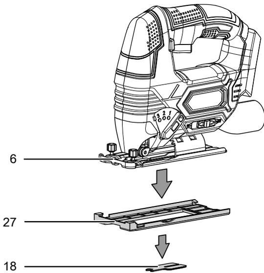
4. To reinsert the anti-splinter guard (18), carefully push it into the recess of the base plate (6) from below until the anti-splinter guard (18) locks in place. When doing so, make sure that the smooth side of the anti-splinter guard (18) points away from the device.
