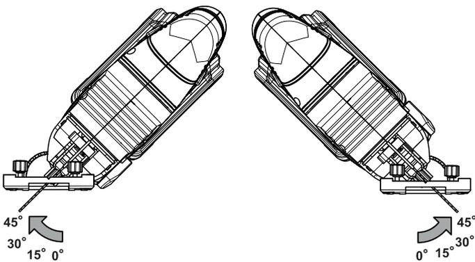
6. Slide the base plate (6) back to the front until the toothing engages.
