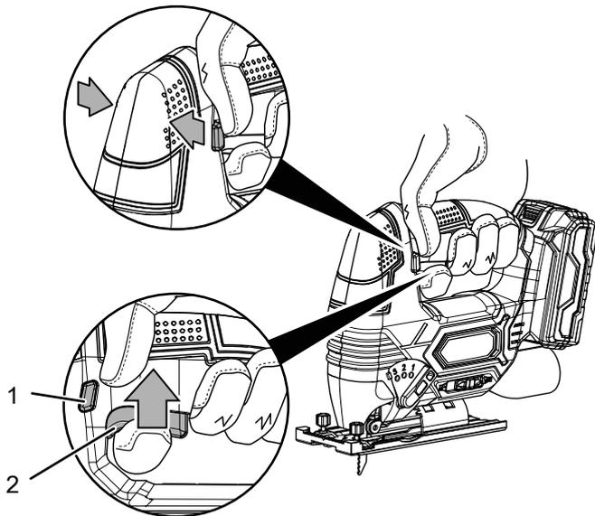
6. Let go of the on-/off-switch (2) to stop the device.
