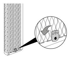
3. Remove the evaporation filter from the holder for the air filter.
