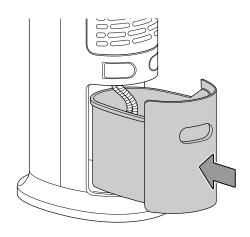
10. Lock the water tank by turning the clip from its horizontal position into the vertical position.
