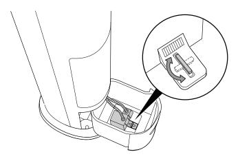
4. Take the pump out of the water tank. While doing this, make sure not to damage or loosen the connected cable or the hose attached to the pump.
