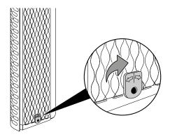
10. Reinsert the air filter into the device.
