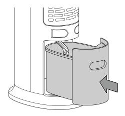
12. Lock the water tank by turning the clip from its horizontal position into the vertical position.
