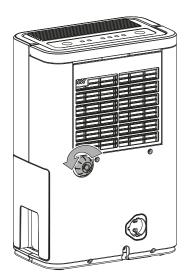
2. Push one end of the hose onto the hose connection.
