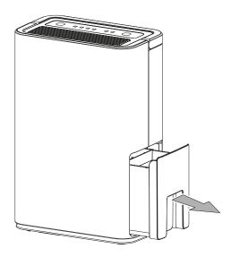
2. Empty the condensation tank over a drain or sink.
