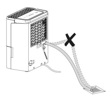
Remove the hose if you want to collect the condensate in the condensation tank again. Allow the hose to dry prior to storage. The hose can be connected in any operating mode for continuous operation.
