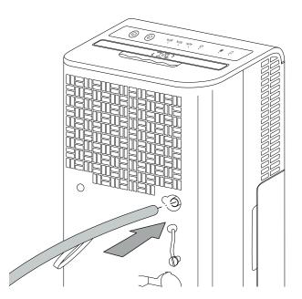
Guide the other hose end to a suitable drain or sufficiently dimensioned collection container. Please observe that the hose must not be kinked.
