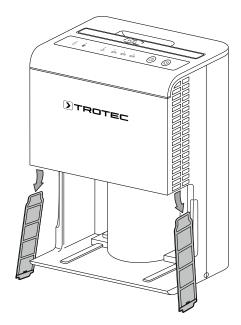
3. Clean the filters using a slightly damp, soft, lint-free cloth. If the filters are heavily contaminated, clean them with warm water mixed with a neutral cleaning agent.
