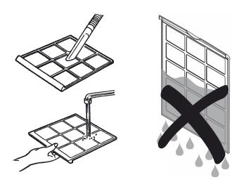
4. Allow the filters to dry completely. Do not put any wet filters into the device!
