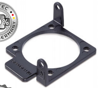
The PlugSafe base plates are designed for built-in sockets with flange mounting. Two opposing, diagonally arranged angle brackets permit the safe application of the socket in accordance with the regulations e.g. by using a consecutively numbered seal. PlugSafe can be used for protection both with an inserted power consumer or when the socket's cover is shut.
