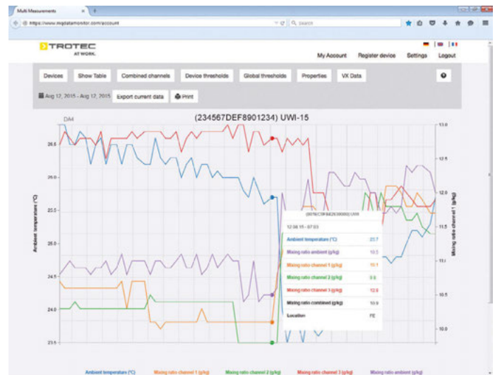
The detailed display contains the drying progress for the selected period of time. An alternative tabular representation of the measured values is also not a problem.
